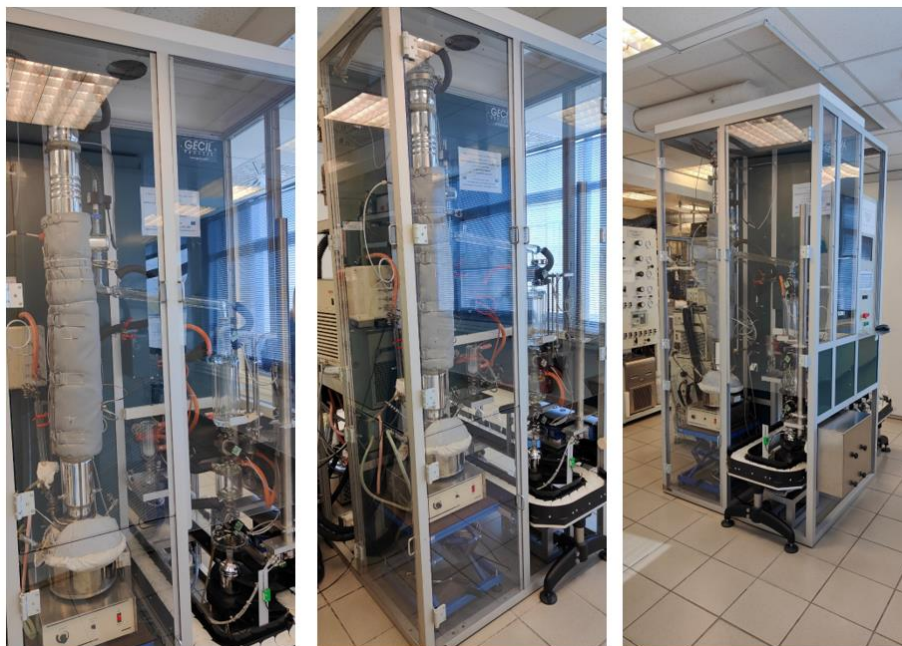
Figure 3: Fully automated lab-scale distillation apparatus at CERTH
